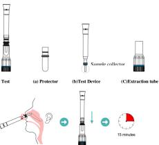
When placing the test device vertically into the extraction tube, the edge of the extraction tube must reach the top of the supporting ring. If not, this may lead to lateral flow failure, resulting in an incorrect result or invalid result.
